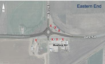
Roundabouts are circular intersections designed to direct movement counterclockwise.
