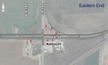
Restricted Crossing U-Turn (RCUT) modifies how side road traffic crosses or turns left at the highway by re-routing left-turn and through vehicles from the side road.
