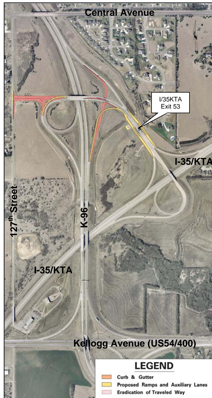
Figure 2.8 Interim Improvements at I-35/KTA Exit 53
